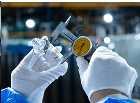
Cold End In-line Random Inspection
