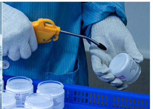
Final Inspection and Dust Removal
